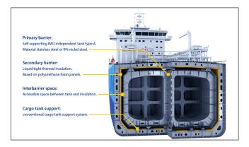
The LNT A-Box is based on IMO independent type A tank design, the simplest configuration according to the IGC Code
