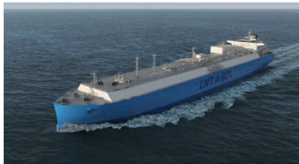
Figure 4. Large scale LNG carrier based on LNT A-BOX.
