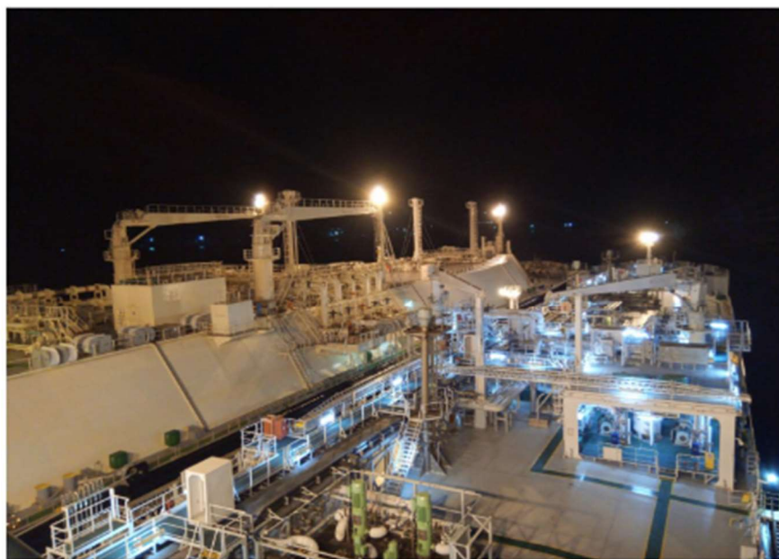
Figure 2. Saga Dawn conducting ship-to-ship (STS) loading from a large scale LNG carrier.
